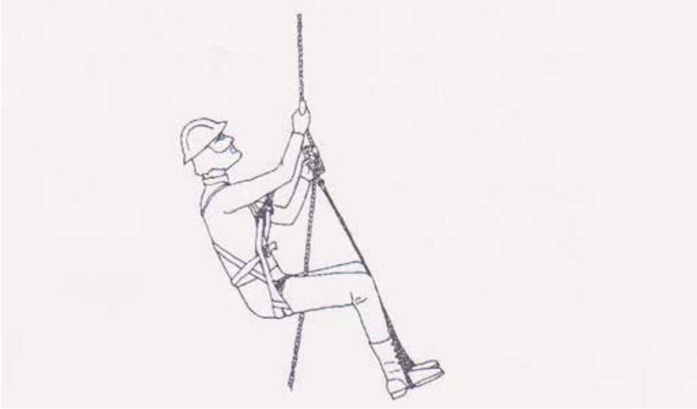
Figure 2. Position of equipment during climbing procedure. The lower ascendor is being lifted to the upper ascendor. Note the strap-type harness which provides cool, comfortable support.
