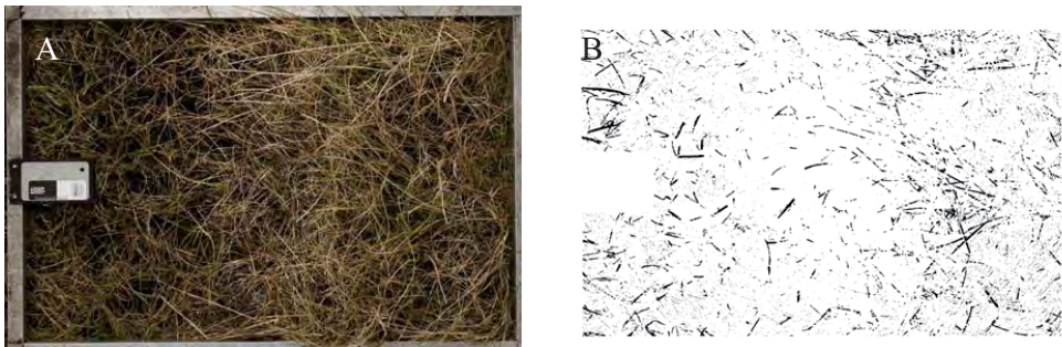
Fig. 5. Thresholded binary image (B) of an image taken in October 2008 (A). The frame and white balancing card was removed before number of green pixels was counted as seen on image B.
