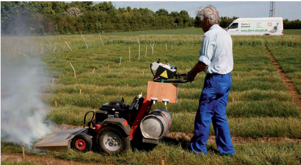
Fig. 7: The gas burner HOAF thermHIT ® 75M that was used in the experiments presented in Paper II and III.
