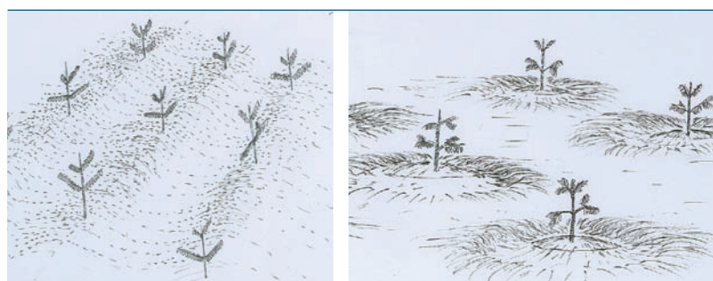
Drainage of vertisols around plants reduces the stress of waterlogging. Left. Planting on ridges between drainage trenches. Right. Circular draining trench around each seedling
